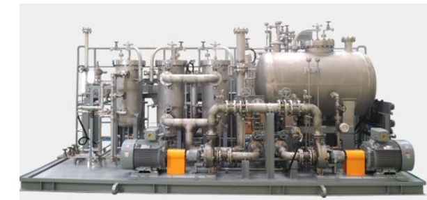
Seal Oil Unit
