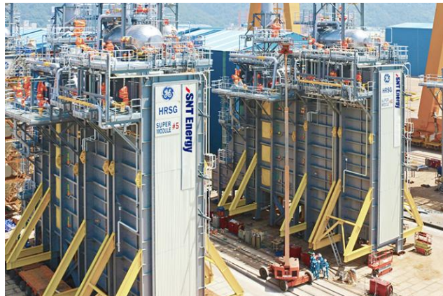
Heat Recovery Steam Generator
